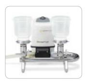
The Microsart® Combi.jet is a 2-branch manifold, made of high-grade stainless steel. The manifold has been specifically designed for the use together with the Microsart® e.jet Transfer Pump. The system is able to create sufficient vacuum for vacuum filtration concomitantly transferring the filtered liquid directly to waste. Microsart® Combi.jet and Microsart® e.jet can be easily connected and disassembled by the innovative Quick Connection technology.
