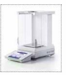
Quality management features take the worry out of weighing and provide you with a high level of trust in your results: the built-in Test Manager keeps routine tests under control, StatusLight gives you the goahead when it's safe to start your weighing tasks, and the electronic LevelGuide ensures your balance is perfectly levelled.
